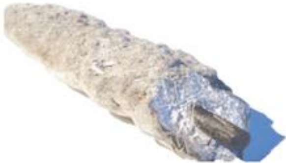
A cross-section of a Biorock structure, nine months after installation.
